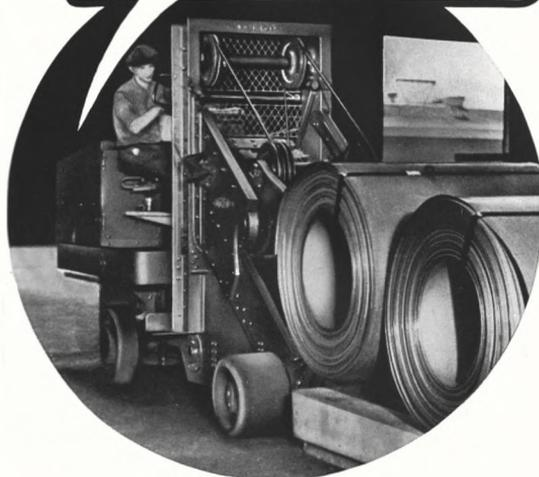
● Edison Batteries thrive on hard work. There are big batteries to do big jobs. The picture above shows an Edison-equipped battery truck which can handle loads up to 20 tons, day in and day out. Ten years ago, in industrial truck service, batteries were seldom called upon to handle more than 2 tons at a time.
